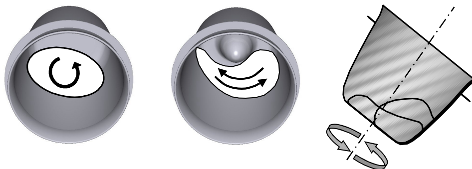
Figure 9 : Mixing efficiencies in flat bottom crucibles and Bis!™ crucibles.
